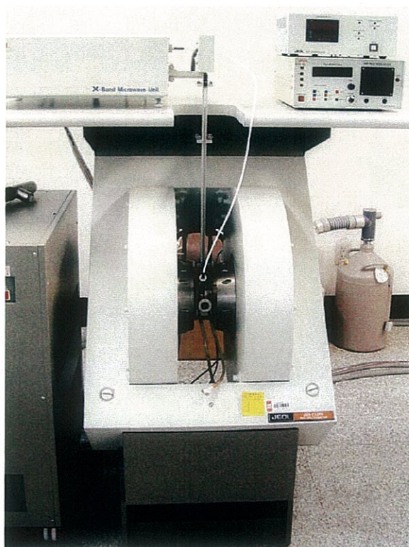
Figure 2. This JEOL FA-300 spectrometer with a manganese marker is the ESR instrument used in the study. Photo by Y. C. Kim.
