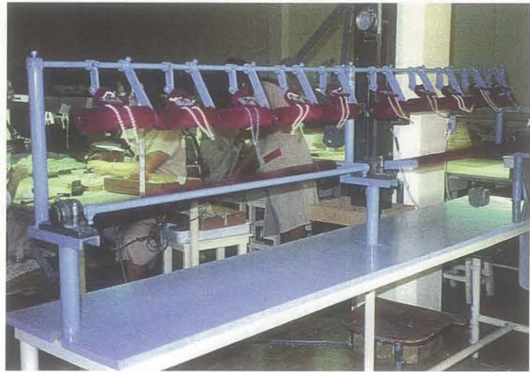
Figure 10. As a final step, selected strands of the finished Majorica beads are subjected to strenuous durability testing. Here, the strands are mounted on a special machine that literally "beats" them against a rotating bar to simulate years of wear. Photo by June Hanano.
