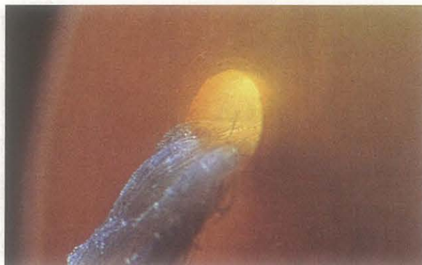
Figure 3. In many of the cultured pearls, the color appeared to be concentrated near the surface when viewed down the drill hole. Such concentrations of color in pearls are good indicators of treatment. Photomicrograph by John Koivula; magnified 5 \times .
