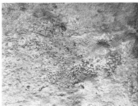
Fig. 1 9 days after operation in July. Showing the dendritic growth of aragonite crystals on a nucleus. \times 270
