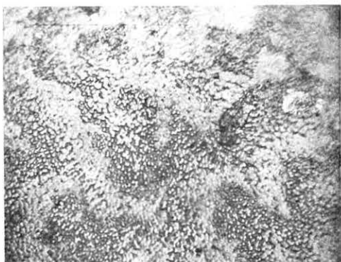
Fig. 7 13 days after operation in September. Showing the aggregates of aragonite crystals developed in step. \times 270
