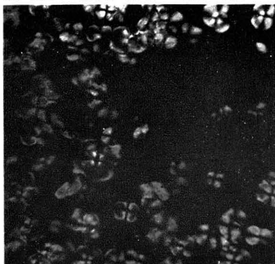
Text-fig.1 Photomicrograph of a thin fragment of prisms grown on a surface of conchiolin membrane. (Crossed nicols). \times 80
